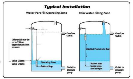
Note: Keep overflow, rain water inlet and outlet to pressure pump as far away from the float valve as possible.
